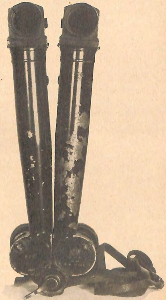
Figure 299. This battery commander's telescope has an 8\times magnification and a 6^\circ field of view. It is constructed so that the telescopic arms may be placed in a horizontal position for better stereoscopic vision.
